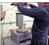
Water/chemical and powder loading into mixing chamber
