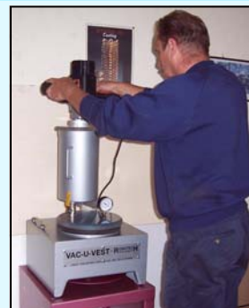
Mixing blade & variable speed motor system, operated by operator holding controls with both hands
