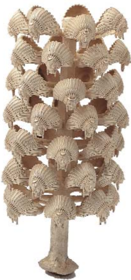
Castings made with the J-2R have better surface quality and detail than castings made with traditional machines.
