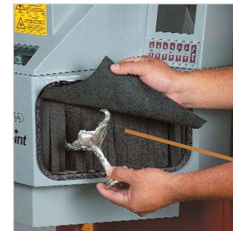
Extra-wide access ports increase maneuverability and allow larger items into the weld chamber for repair.
