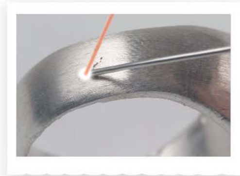
Correct surface porosity with wire filler.
